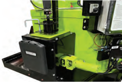
External heated 20 gpm material pump
