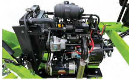
19hp Isuzu tier IV diesel power plant
